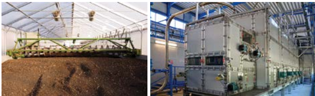
Figure 7: Solar drying in greenhouses (left) and thermal dryer (right). Credit photo: suzewatertechnologies.com
