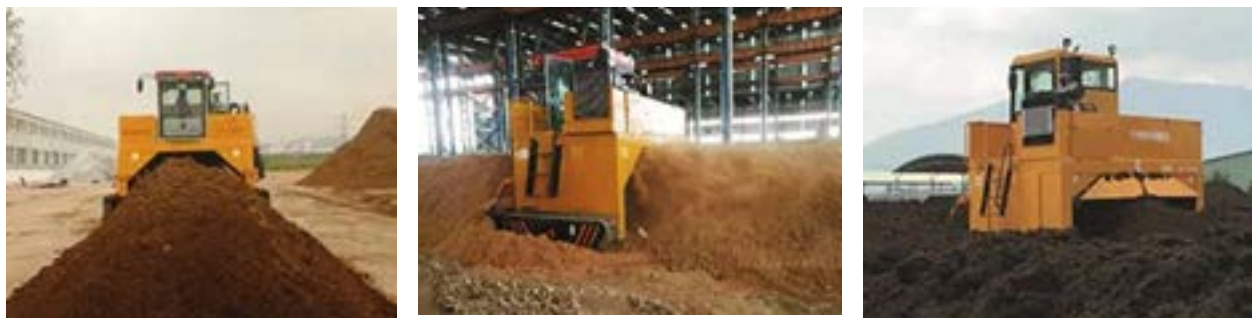
Figure 5: Sludge composting using a compost turner, which allows maximum space utilisation at the composting site. Photo credit: cnhydraulicpress.com/
